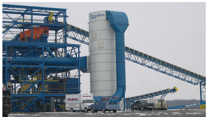
780LP12 at Coal Classifying Plant 75,000 cfm (127,339 m 3 /h)
