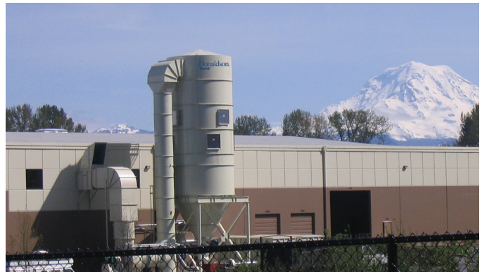
528LP12 at Cabinet Factory 70,000 cfm (118,906 m 3 /h)
